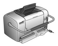
6. Set the cartridge lock lever in the Release position by sliding the lever to the right, then down and to the left. The photo cartridge will be ejected about halfway out of the holder. Pull the cartridge out of the printer and dispose of it properly.
